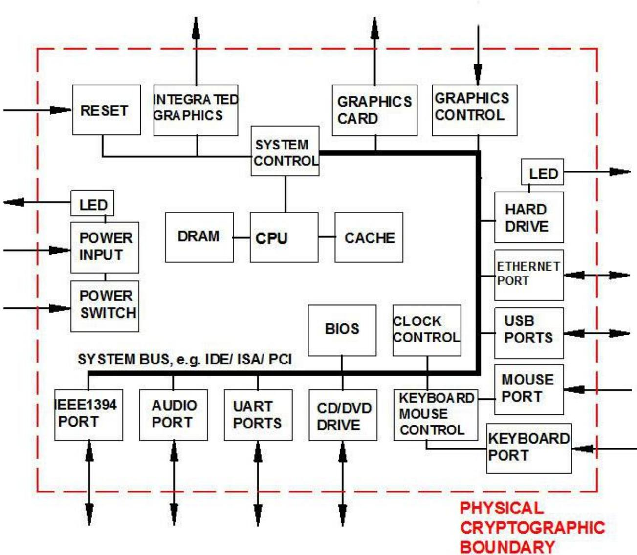
For FIPS 140-2 purposes, the BC-FNA Module is defined as a “multi-chip standalone module”, therefore, the module’s physical ports or interfaces are defined as those for the
